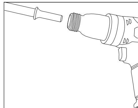
3. Screw the spring retainer onto the cylinder by turning the top hook in a clockwise direct. Make sure the spring retainer is firmly secured.
