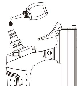
3. After adding oil, connect the tool to the air source, run tool briefly. Wipe off any excess oil from the cap exhaust.
